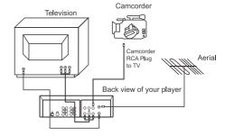
If you have connected your camcorder in this way, you can also connect a RCA lead from "AV" on the back panel of the player to the television. To use this function, you can also connect the camcorder by using a phono cable if your player has front input sockets. Check the front of your player for this connection.
